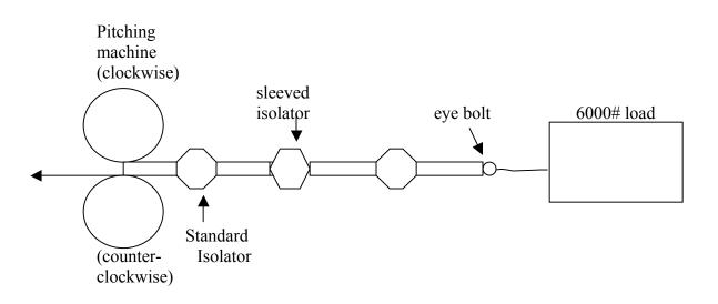
After the initial tests, we will run additional tests if necessary based upon the initial test results. The variables that can be adjusted are the pitching machine wheel pressures, distance between wheels, and the wheel rpm and torque.
